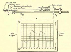
Fig. 59.—Method of setting planimeter so that it will read the mean or average height of graph.
